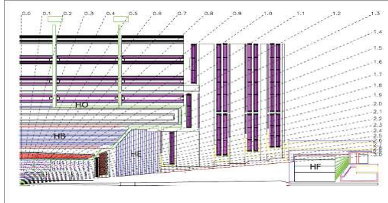
Sq'hma 2.5: Cross-section of one quadrant of the hadronic calorimeter.
